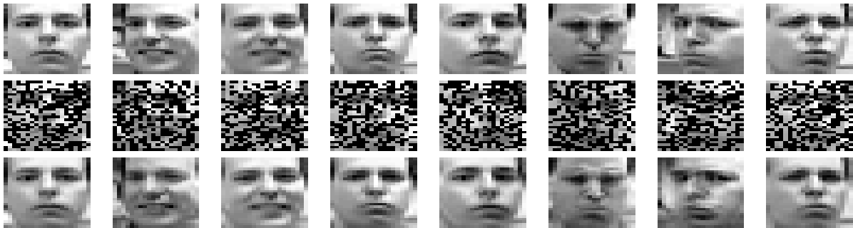
Figure 2: Examples of reconstruction of partially observed test images in Frey faces by applying the Bayesian GP-LVM. Each column corresponds to a test image. In every column, the top panel shows the true test image, the middle panel the partially observed image (where missing pixels are shown in black) and the bottom image is the reconstructed image.
